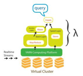
Fig. 3. REAλICS Lambda based configuration. Tools from the Cloudera Hadoop ecosystem are placed in the corresponding layers of Lambda. The tools outlined in this figure are only indicative
